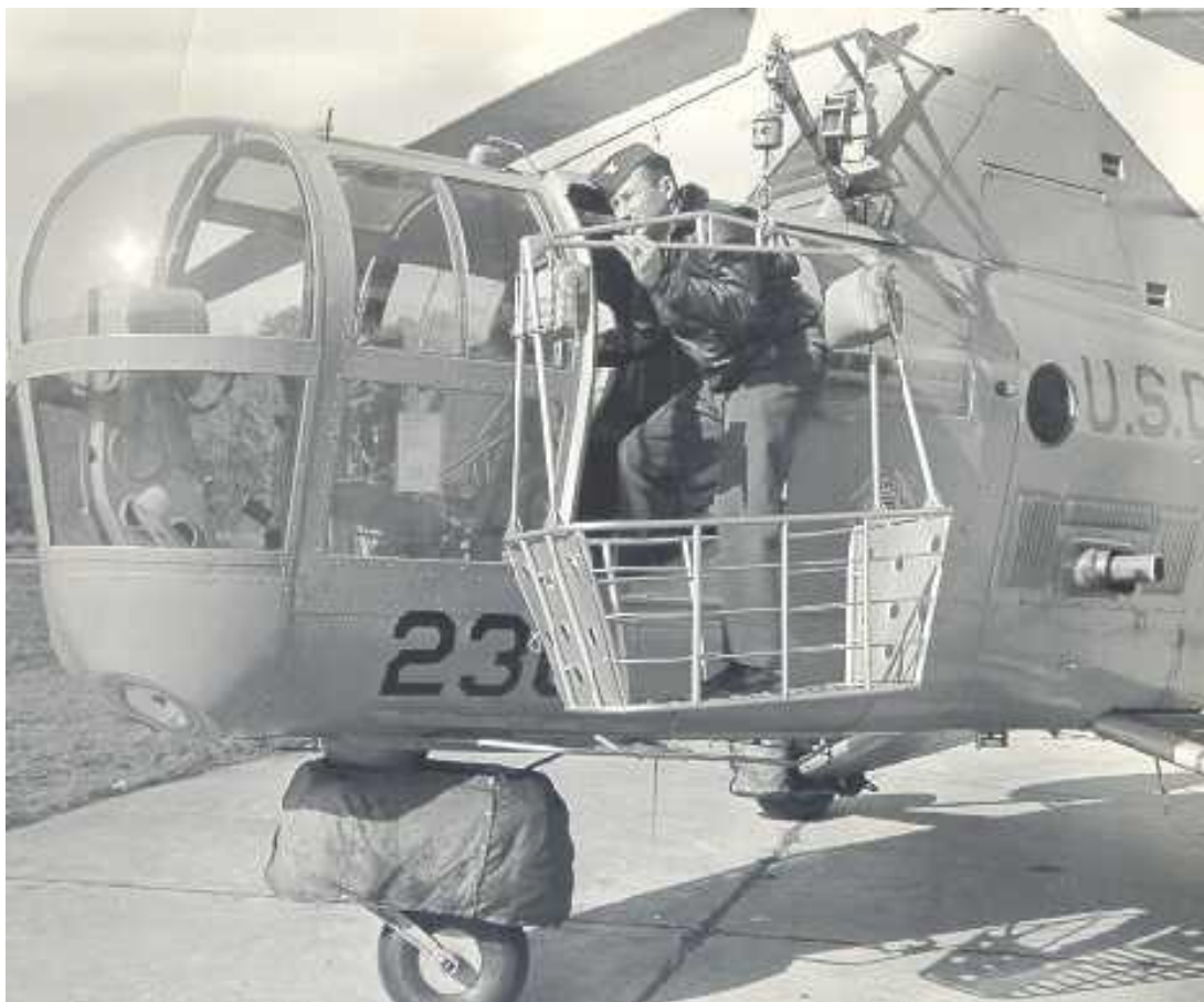
LT Stew Graham at the hatch of a HO3S with a rescue basket attached to the hoist. With the advent of the HO4S the basket could be brought inside the cabin.
