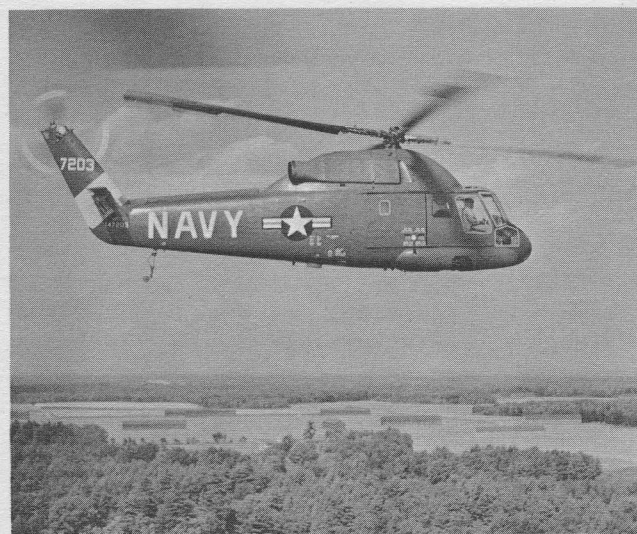
HU2K-1 — The U.S. Navy's new high speed, all-weather helicopter. The aircraft is powered by a T-58 Turbine Engine.
