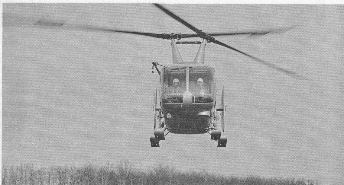
This head-on view shows the synchropter design and features of local base rescue configuration of the HUSKIE.
