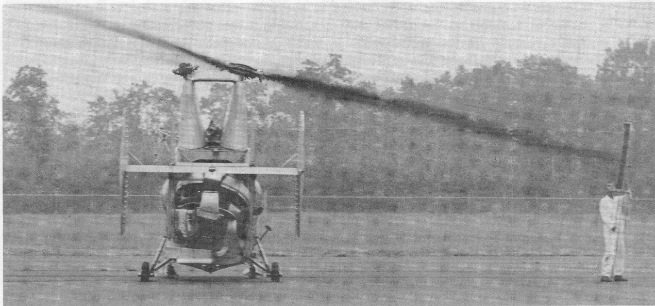
PICTURED IS A DEMONSTRATION of an H-43A showing blade tracking procedure with use of the tracking flag. Note adequate clearance to the side of helicopter when parked on level, hard surface. The mechanic shown is a six footer.
