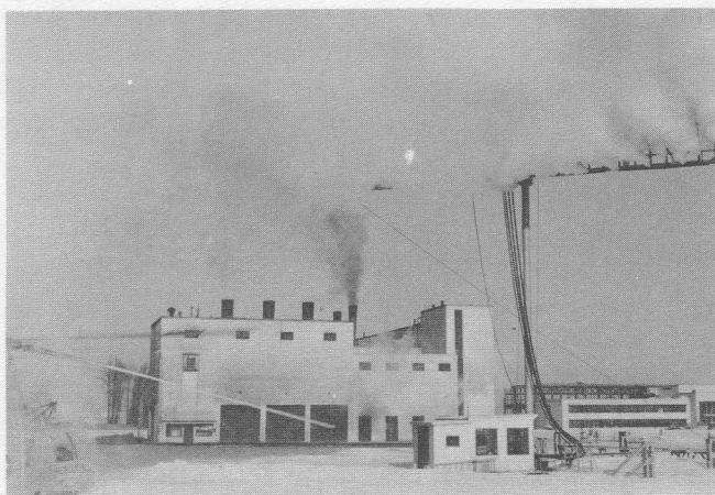
ARTIFICIAL CLOUD PRODUCER is this test icing facility, left, constructed by the Canadian National Research Council at Uplands Royal Canadian Air Force Base, Ottawa, Ontario. At right, H-43B Huskie is almost obscured by whirling snow as it turns up preparatory to entering icy cloud at test rig.
