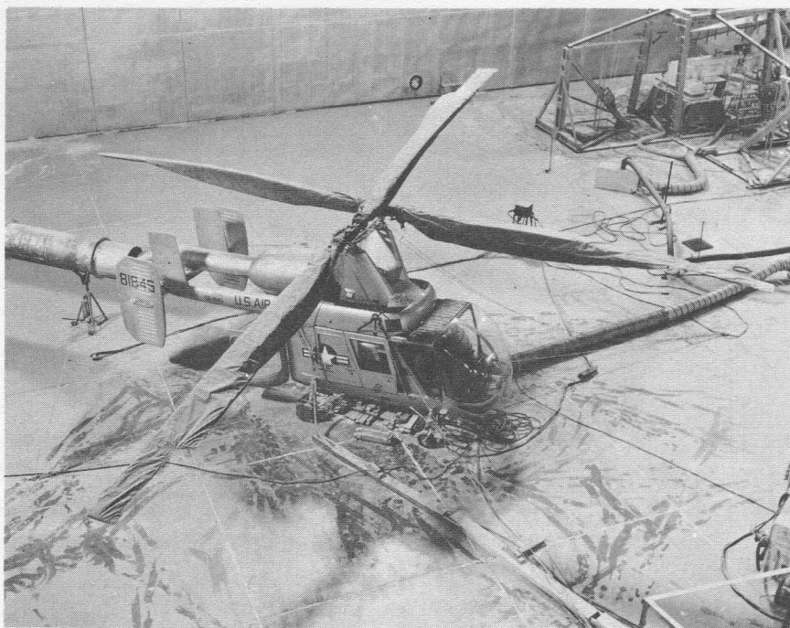
THE HANGAR TEMPERATURE has been dropped from +70° down to 0°, then -25° and finally to a cold, cold -65°F. Test engineers, not anxious to contract a case of frostbite in sunny Florida, have retreated to the heated booth positioned nearby. This serves as the control center for the test operations conducted after a minimum cold soak period of 24 hours.
