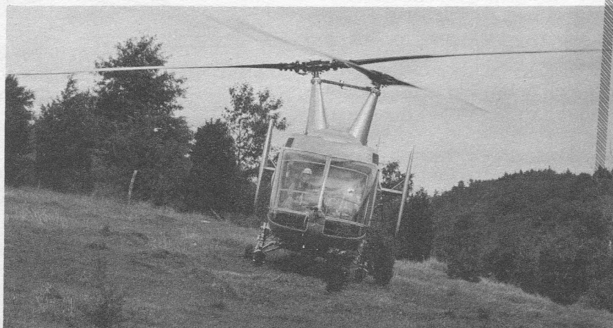
LOW EXTENDED PRESSURE of the Huskie strut design is shown in this view of a sidehill landing. The first weight of the helicopter has compressed the uphill strut while the downhill strut is still only partially compressed, thus keeping the angle of inclination to a minimum.
