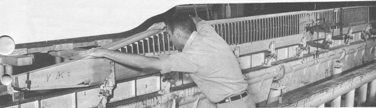
CRAFTSMAN AT WORK —This rib-bonding fixture holds and locates ribs, spar and trailing edge spline during bonding operation.
