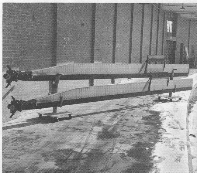
LATEST BLADES —Development by KAC of these glass fiber helicopter blades marks a significant advance in resistance to rotor blade fatigue and makes possible major savings in manufacturing and maintenance costs.
