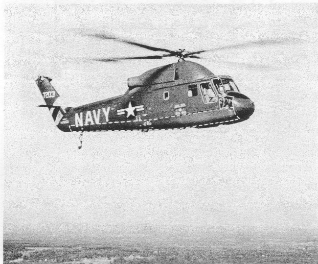
HU2K-1'S WATERTIGHT COMPARTMENT and flotation gear are located in area indicated by broken white line.
