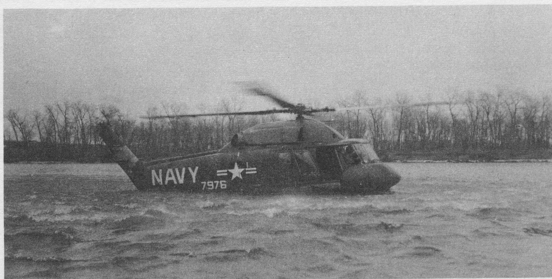
HU2K-1 LANDS ON CONNECTICUT RIVER and begins taxi tests to evaluate maneuverability of the helicopter with flotation bags inflated.
