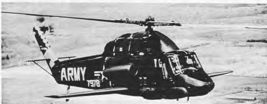
**WINGED SEASPRITE** — Kaman's 200-mph-plus UH-2 experimental helicopter with jet engine mounted on side and pair of wings added.
