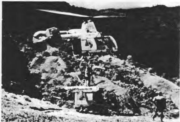
**HUSKIE WITH THE HUSKIE** — Problem of recovering HH-43B downed in rugged Colombia, S.A., terrain after roll-over accident is easily solved by utilizing another HH-43B to remove fuselage and other components. Both aircraft are attached to the Colombian Air Force.
