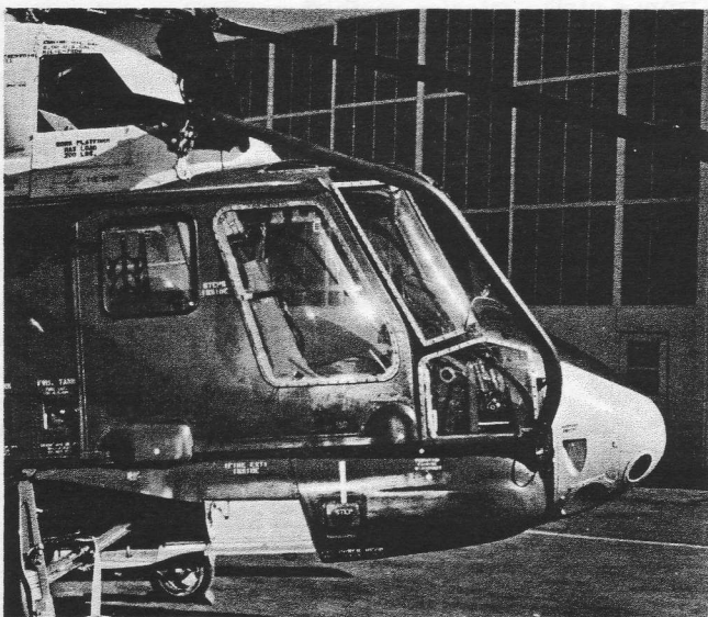
Fishpole Boom — Boom on UH-2 is shown in stowed position with hoist hook suspended over the rescue door.
