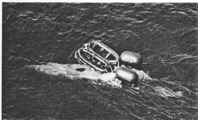
READY FOR SALVAGE —With step 1 of POSITION B accomplished, this downed bird is ready for a salvage crew to start the righting sequence which will eventually return the aircraft to service. (USN photo)
