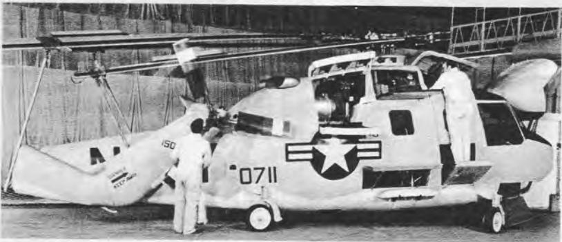
**Maintenance**—Major emphasis has been placed on ease of maintenance. All SEALITE equipment is accessible through quick opening access panels, many of which also serve as work platforms. At right, a single ground support tool attaches to hardpoints on the aircraft and permits rapid removal of the engine (s), rotor or transmission either in the hangar or on deck.
