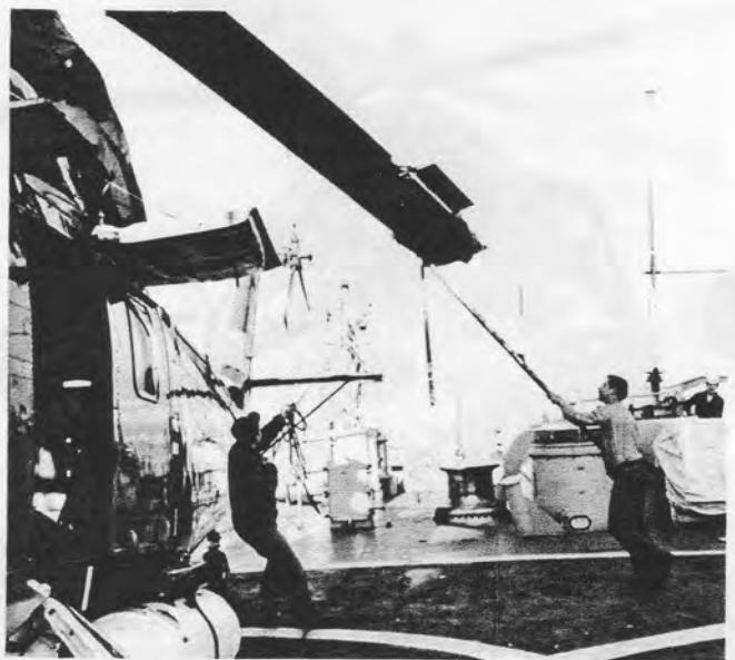
**"Snoopy's" Keepers**—Photo above, easy goes it as a main rotor blade is folded for the day. It's a handy convenience when there is a space shortage. Left photo, ADJ3 Lemay inspects a pitch change link on the tail rotor—a rotor that takes a lot of punishment during day-to-day operations (1679 RPM).
