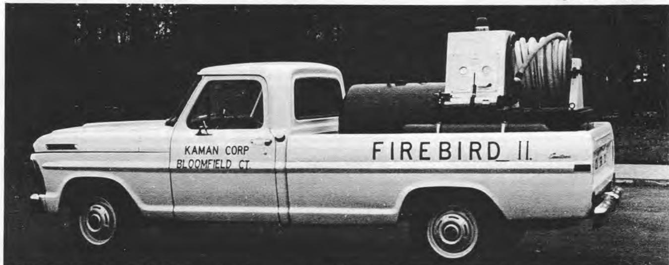
**Firebird II—Truck Mounted**—A winterization kit is available which makes the Firebird self sufficient in any weather to -20°F.
