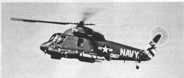
New Role For SEASPRITE —Top view shows SH-2D with MAD gear mounted on right side. Note radome under nose of aircraft, just forward of main landing gear. Bottom photo shows helicopter with torpedo installed.
