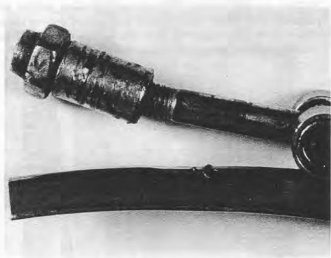
"More Vee-band couplings are damaged because of over-torque." The T-bolt shown in the Photo is an example of what occurs when too much torque is applied. This coupling, acceptable in all other respects, must be rejected because of an installation error.
