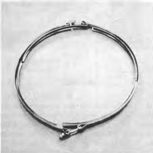
The Photo shows the V-band used to secure an H-2 engine bellmouth. The V-band utilized on the engine exhaust is also of the two-bolt type but it is of a heavier construction. The two or one bolt type V-bands can be installed by following the instructions detailed here. One bolt vee bands are usually found on small diameter installations.
