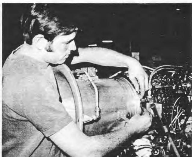
"Under no circumstances should the coupling support the bellmouth assembly until the installation has been completed." Damage to the V-band will result if the bellmouth is allowed to "droop" and apply a load on the V-band. The mechanic in the Photo is using his body to press the bellmouth against the engine inlet while initially engaging the T-bolt. He will then gently move the bellmouth while alternately tightening first one nut and then the other.
