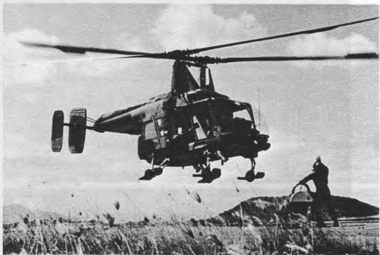
**Training**—In top left photo, HH-43 crew uses a rescue basket during a practice mission. The device may be used for land or sea pickups and also as an auxiliary stretcher. In right photos, Det 1 crew practices hookups with simulated fire suppression kit; HH-43 "Pedro" takes aboard a simulated survivor. (USAF photos by Amn Randy W. Day)
