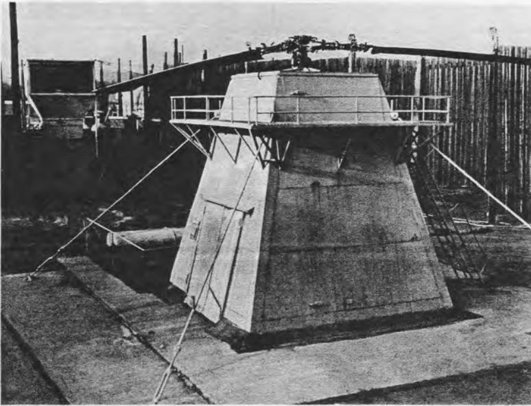
**TEST RIG**—The 101 rotor blades and controls are shown on one of the Kaman whirl rigs at the Bloomfield, Conn., facility. On the rigs, production blades are matched with a master blade before delivery to military customers. Experimental rotor systems are also tested in this area. At left is a rectangular viewing window which incorporates mirrors to observe test blade operation from the safety of the concrete "blockhouse" beneath. (Ruggiero photo)
