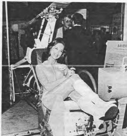
Continued development and refinement of the folding, telescoping rotor system on the Kaman SAVER rescue ejection seat are provided under an approximate \$100,000 contract recently awarded by Naval Air Development Center, Warminster, Pa. The modifications are intended to enhance consistency of performance during SAVER's rotor deployment and lead into the next phase of the unique vehicle's development-transitional deployment of the entire system in unmanned air drop tests.
