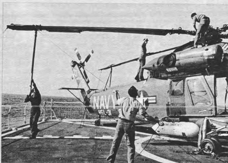
Unfolding the helicopter blades in preparation for a flight are left to right on deck, AMS3 Williams and AT2 Gunter. On the aircraft, left to right, are, AMS3 Henningfield and AMH2 Douglas R. Colwell.
