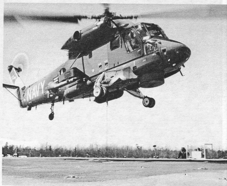
TESTING BEARTRAP —An SH-2F LAMPS helicopter at the Naval Air Test Facility's new Helicopter Support T&E Center is shown during testing of the "Beartrap" haul-down and securing system. (USN photo)
