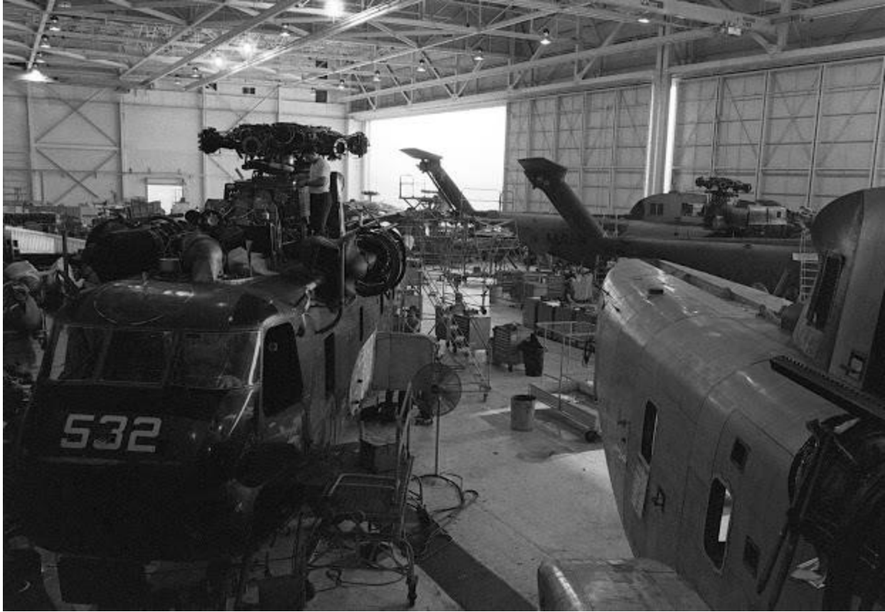
CH-53 Sea Stallion helicopters undergo sheet metal maintenance and repair at the Naval Aviation Depot, NAS Pensacola, Florida, in 1989. ( Jerry Antone/ RG 330, National Archives )
