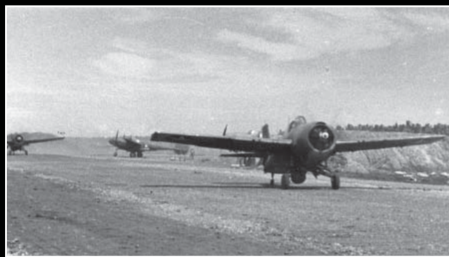
Marine F4F-4 Wildcats and Army Air Force P-38 Lightnings taxi out for takeoff on Guadalcanal. Closest aircraft has a field-mod 42-gal centerline drop tank, while the next Wildcat has a wing mounted tank, starboard side only. (NMNA)
