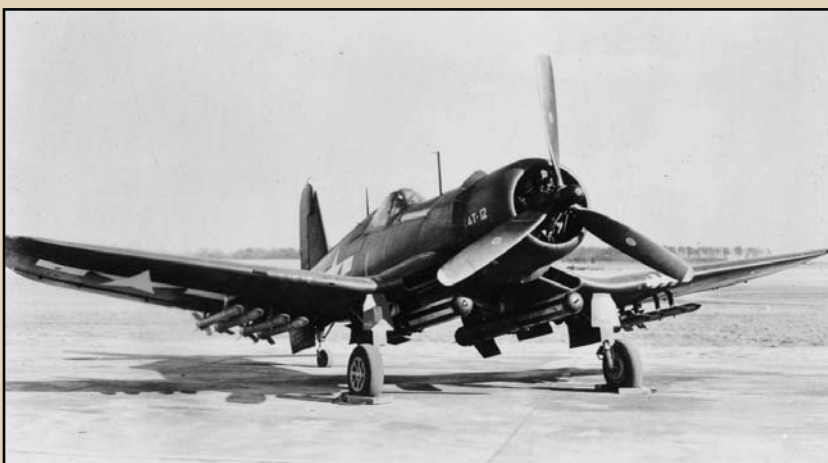
This Chance Vought F4U-1D is equipped with two 11.75-inch "Tiny Tim" air-to-ground rockets. Tiny Tim was used operationally at the end of World War II and later in Korea. Had Project DANNY been carried out, it would have been the only use of Marine Aviation in the European Theater of War during World War II. (Tom Doll Collection)
