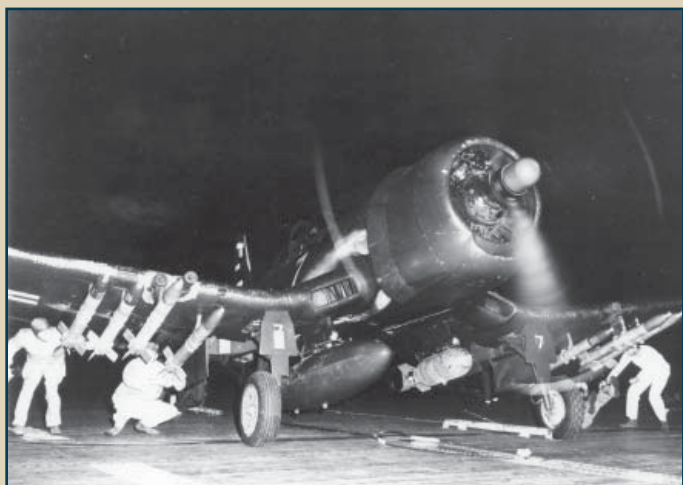
Preparing for night operations, ordnancemen secure arming wires to 5-inch rockets on this VMF-214 Chance Vought F4U-4 Corsair. CAPT Thach’s USS Sicily (CVE 118) and her embarked Marine aviators provided crucial Close Air Support in the opening weeks of the Korean War. (NHHC)
