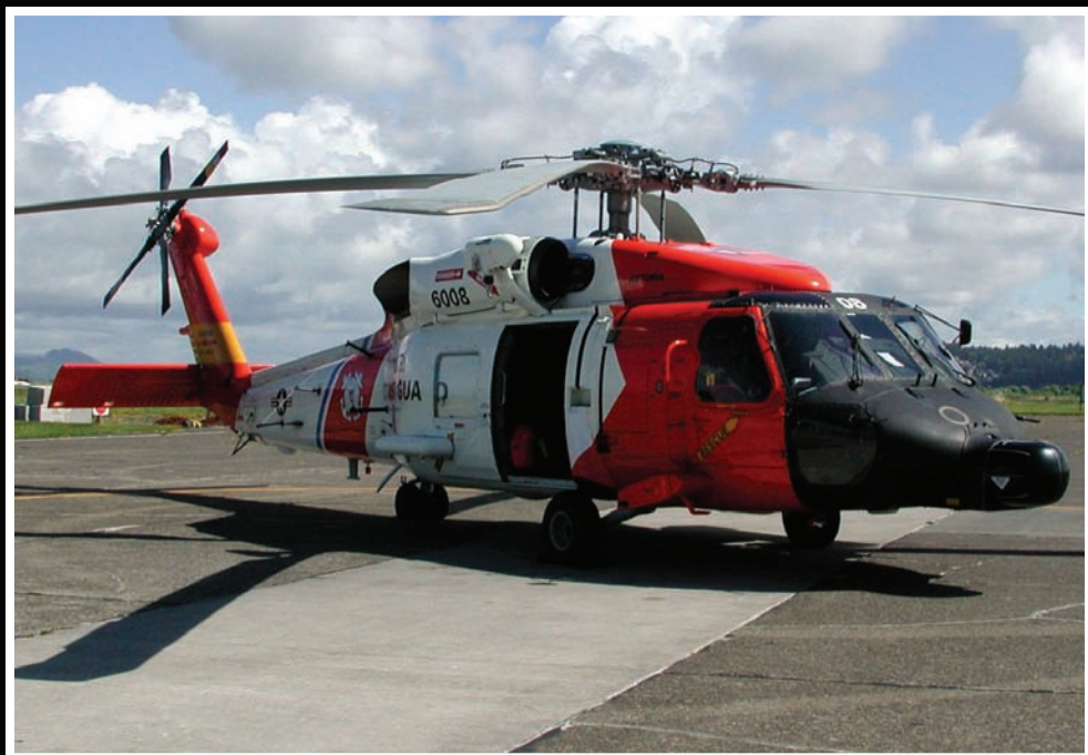
Sikorsky HH-60J Jayhawk (6008) on the ramp at CGAS Astoria, Oregon. 42 Jayhawks were built and the Coast Guard is currently upgrading the airframes to the MH-60T configuration. (USCG)
