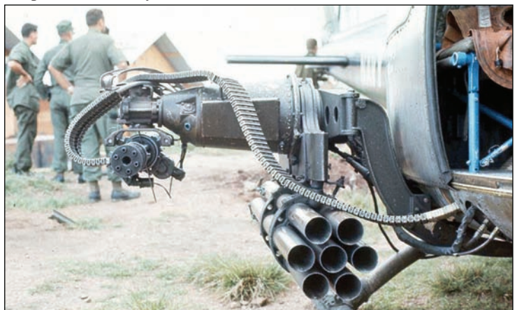
The business end of a Seawolf Huey. The aircraft is equipped with a 7.62 mm Gatling gun and a seven-shot 2.75-inch rocket launcher. (Courtesy of Tom Phillips)
