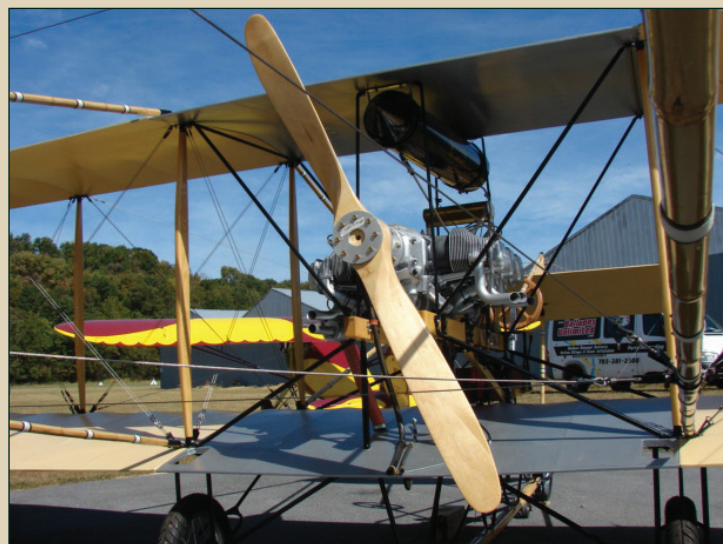
Bob Coolbaugh's Curtiss Pusher is powered by a Continental C-125-2 six-cylinder 125hp horizontally opposed engine for greater reliability and safety. (Bob Coolbaugh)
