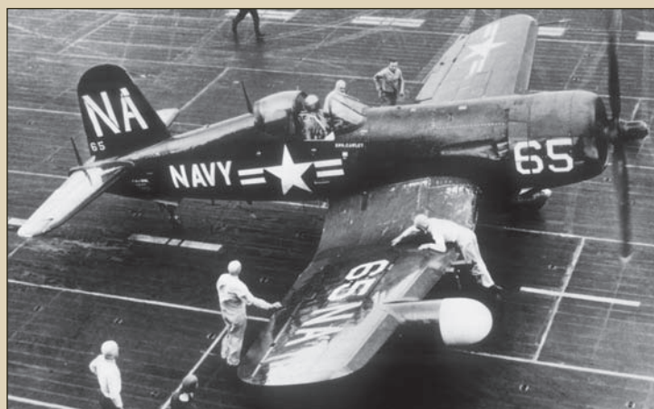
F4U-5NL (BuNo 124511) of Composite Squadron FOUR (VC-4) prepares for launch. De-icer boots are plainly visible on the wing leading edges. (Vought Heritage Group)
