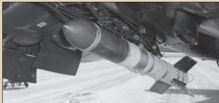
A “Tiny Tim” 11.75-inch rocket installed on the centerline rack of an F4U-1D Corsair. (Gary Verver Collection)
