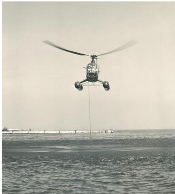
XHOS with Sonar transducer under water
