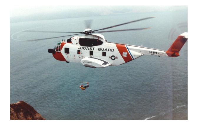
In November 1967 the US Coast Guard procured the first of the HH-3F Pelican Helicopters. This twin turbine, medium range, amphibious, all weather helicopter extended the Coast Guard offshore search and rescue capabilities. The HH-3F had a maximum speed of 142 knots with a normal cruise speed of 130 knots and a range of 650 NM. The Coast Guard purchased 40 HH-3F's. The last one was delivered in 1973.
