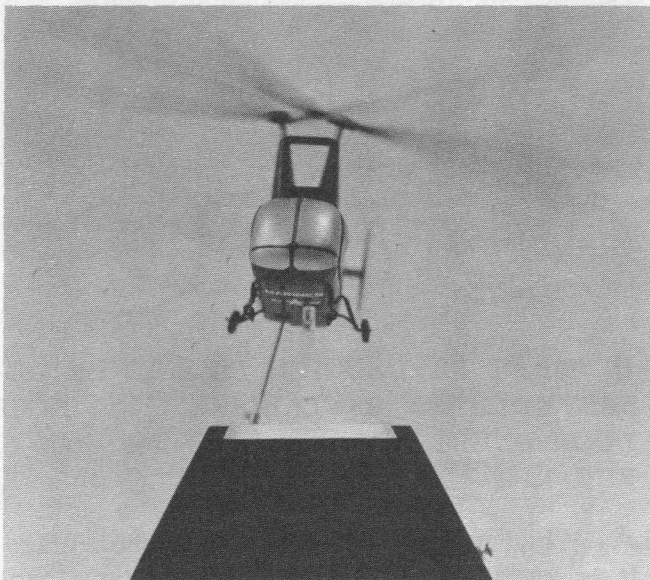
ED WHITE, KAMAN FIELD SERVICE REPRESENTATIVE IN JAPAN, uses this "energized" model of an HOK-1 while explaining how the synchropter design works. White used a small, battery-operated motor working through the transmission from a child's toy to power the rotors.
