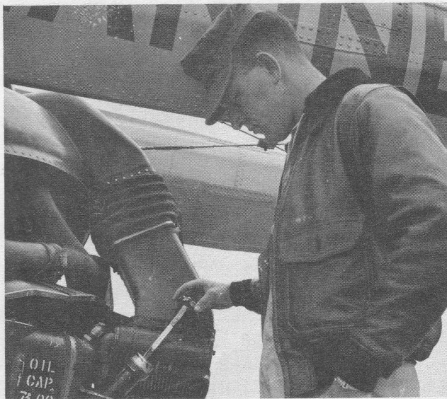
CHECKING THE HOK'S seven gallon oil tank is part of the chief's preflight inspection.
