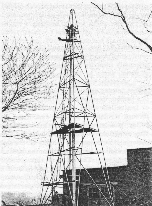
SHOWN IS THE initial apparatus built for internal shot peening of the HU2K-1 blade spar. The spar, which is visible in the photograph, is raised and lowered over rotating internal nozzles. This equipment has since been refined and enclosed in a building, but the original concept is unchanged.
