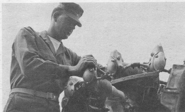
LIKE THE M-1 RIFLE , an HOK's 500 hp Pratt and Whitney radial engine requires periodic and thorough inspection.
