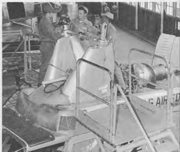
ROTOR HEAD REMOVAL —A2C Marcus, Portland Intl. Aprt., Ore.; A1C Alexander, Charleston AFB, S.C.; SSgt. Washington, Instructor. (USAF photo)
