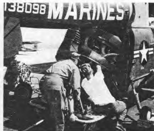
EASY —The exposed engine of the HOK made inspection and maintenance simple for these VMO-mechanics.
