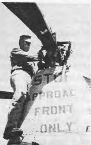
HAZARDOUS SAND —Inspecting rotor heads for desert sand is Pfc Russell A. Creamer, HOK plane captain from San Leandro, Calif. Exposed parts had to be wiped clean before each flight.
