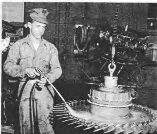
REQUIRED CLEANING —The desert operations made complete engine cleaning a necessity. Here, Pfc Benjamin F. Higginbotham, Little Rock, Ark., cleans the HOK fan and clutch assembly with solvent.
