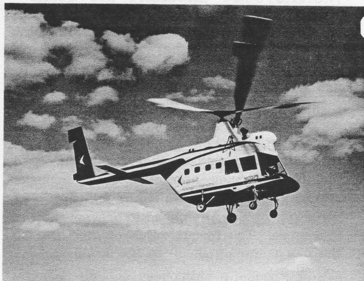
The Kaman HUSKIE III with its twin-turbine engine locations clearly visible is pictured above in flight. The movable vertical and horizontal stabilizer surfaces are also visible.
