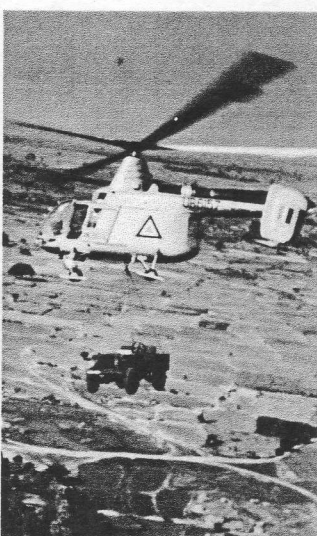
AERIAL DELIVERY —HH-43B's of the Burmese Air Force practice cargo hook utilization with jeep and field gun. Transporting of these and similar loads are a daily occurrence in Burma despite high ambient temperatures and elevations.
