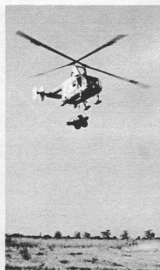
AERIAL DELIVERY —HH-43B's of the Burmese Air Force practice cargo hook utilization with jeep and field gun. Transporting of these and similar loads are a daily occurrence in Burma despite high ambient temperatures and elevations.
