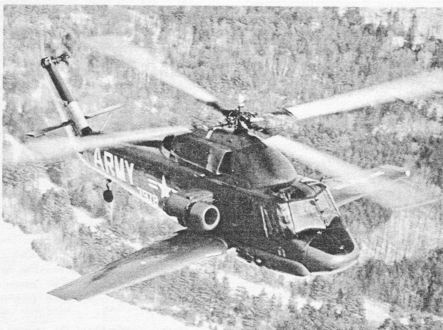
RESEARCH VEHICLE —Kaman "Compound Helicopter" on test flight near the company's Bloomfield, Conn., facility.
