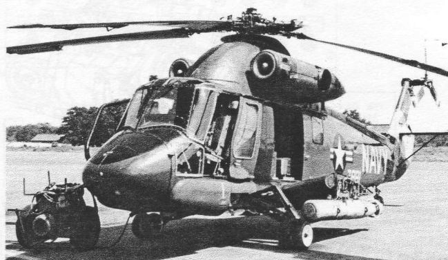
MODIFIED TWIN —UH-2C with range-increasing stub wings is shown on the line prior to testing torpedo-carrying capability. Other offensive weapons were also installed on the helicopter during Kaman stub-wing evaluation.
