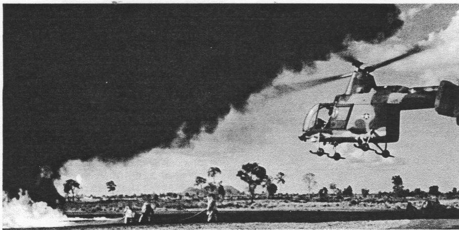
TAKHLI RTAFB (MAC) —Smoke billows from blazing jet fuel while firemen, using a fire suppression kit, extinguish the flames. An HH-43B HUSKIE rescue helicopter from Det 2, 38th ARRS (MAC), hovers behind the firefighters. The rotor blades supply a blast of cool air that protects the firemen. In an actual emergency this procedure is used to rescue trapped crewmembers from the burning aircraft. (USAF photo by A1c Robert W. Hollis)
