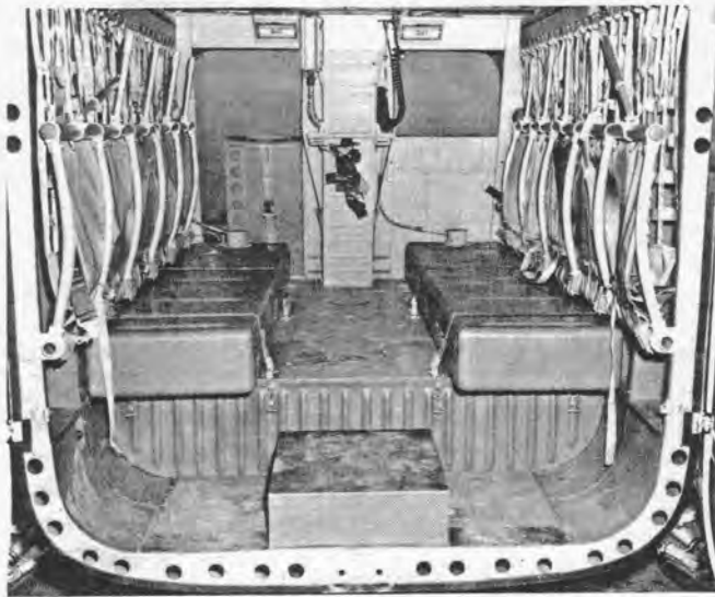
HH-43 AUX FUEL TANKS —Top photos show auxiliary fuel tank installation with troop seats in place and with seats raised. Removal or installation of each tank can be made by two men in five minutes. Third photo shows easily accessible fuel filler cap.
