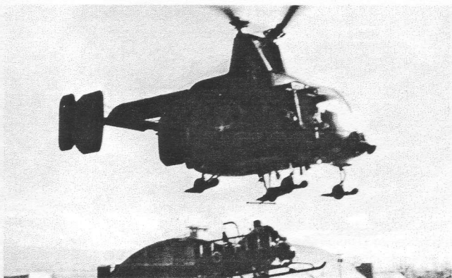
DA NANG (7AF)—ON ITS WAY—A Det 7 HH-43 lifts off with the fire suppression kit to intercept an aircraft which has declared an airborne emergency. (USAF photo by Sergeant Jim Lester)
