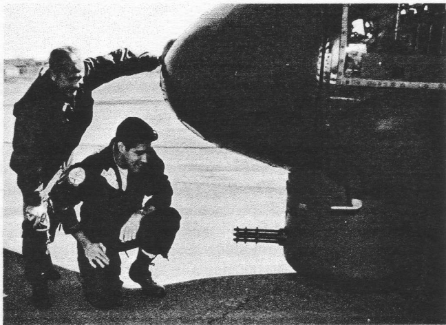
HH-2C AT NAVAL TEST CENTER —The Kaman HH-2C search and rescue Navy gunship is now undergoing testing at NATC, Patuxent River, Md., before its introduction into the Fleet. Starting with a "growth" UH-2C SEASPRITE, the twin-engine helicopter has been fitted with a 7.62mm minigun in a chin-mounted turret, waist-mounted machine guns, and armor. The growth features include an up-rated main transmission, dual wheels and four bladed tail rotor which permit operations at 12,800 pounds gross weight. The Navy has ordered six UH-2C's retrofitted to HH-2C's. The first gunship, above, was flown to the Test Center from Kaman's Bloomfield, Conn., facility by Lt Arthur D. Schatz, USN. Lieutenant Schatz, right, is a WEPTASK pilot from the Service Test Division at Patuxent. With him is Jack C. Goodwin, assistant chief test pilot at Kaman.
