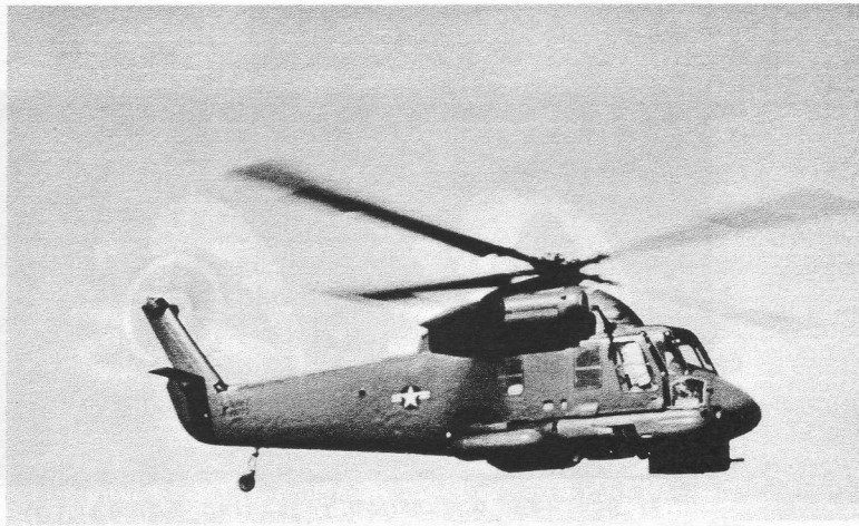
HH-2C AT NAVAL TEST CENTER —The Kaman HH-2C search and rescue Navy gunship is now undergoing testing at NATC, Patuxent River, Md., before its introduction into the Fleet. Starting with a "growth" UH-2C SEASPRITE, the twin-engine helicopter has been fitted with a 7.62mm minigun in a chin-mounted turret, waist-mounted machine guns, and armor. The growth features include an up-rated main transmission, dual wheels and four bladed tail rotor which permit operations at 12,800 pounds gross weight. The Navy has ordered six UH-2C's retrofitted to HH-2C's. The first gunship, above, was flown to the Test Center from Kaman's Bloomfield, Conn., facility by Lt Arthur D. Schatz, USN. Lieutenant Schatz, right, is a WEPTASK pilot from the Service Test Division at Patuxent. With him is Jack C. Goodwin, assistant chief test pilot at Kaman.
