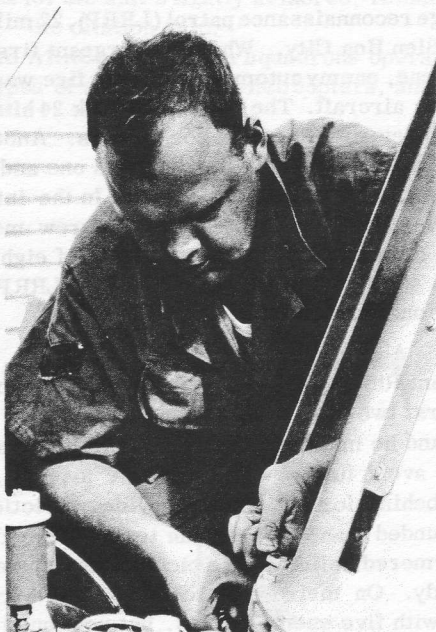
UPTIGHT —Sgt Thomas E. McKittrick adjusts torque on the mounting bolts of the HH-43 rescue helicopter's rotor shaft and housing assembly.
