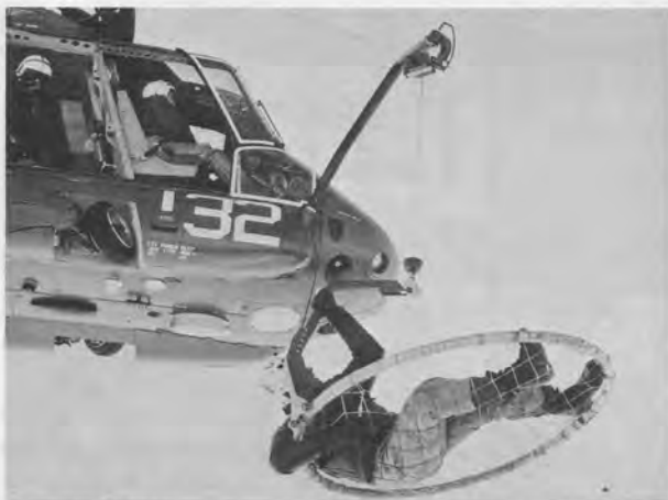
Boom And Net —This dramatic photograph of a UH-2 plainly shows the Kaman-developed fishpole boom and rescue net.
