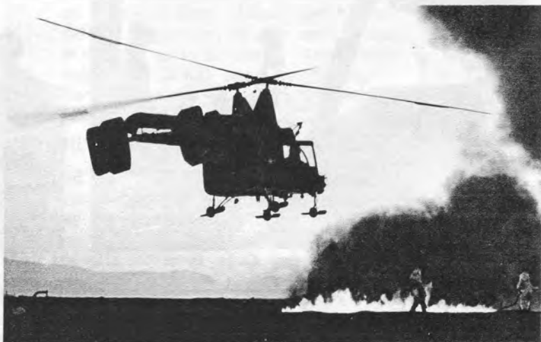
TEAMWORK —Airborne firemen from the 12th Civil Engineering Squadron, aided by the Pedro hovering overhead, hose a path through the flames. The helicopter-delivered FSK, barely visible at lower left, supplies the protective foam used on the fire. The rotor wash from the HH-43 aids firemen in clearing a path and also supplies them with cooling air.
