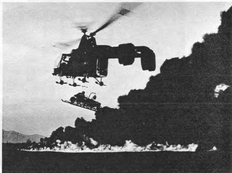
FSK DELIVERY —After picking up the fire suppression kit, the HH-43 hovers near the just-ignited practice fire pit.
