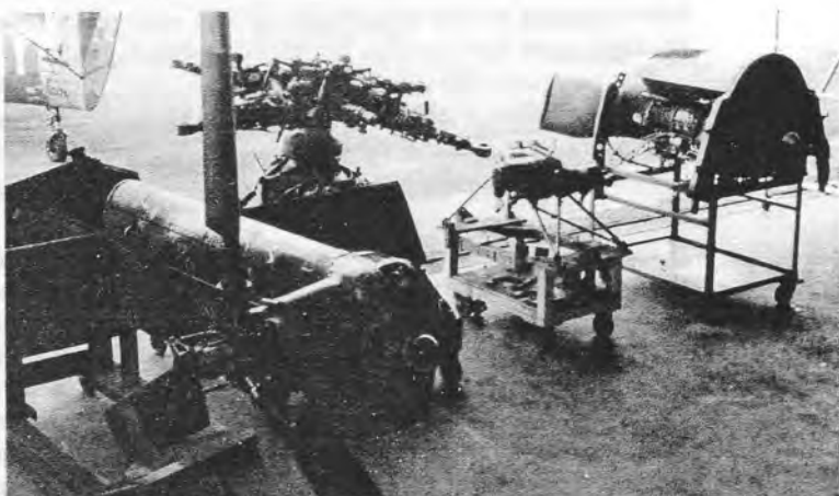
SHOP READY —Pylon, main transmission, hub and retentions, accessory gearbox, and engine unit before entering feeder shops where PAR and modification work will be done. All major assemblies are removed intact.
