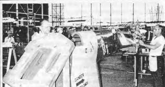
MECHANICAL BUILDUP OF PYLON —Mechanic on left is connecting tail rotor shaft to coupling on the intermediate gear box. Mechanic on the right is installing the four tail rotor blades to the uprated tail rotor gear box.
