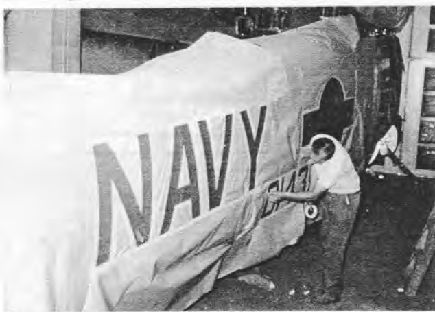
PAINTING —Navy insignia in process of being masked for final spraying. This is one of 260 external markings which will be applied. As a note of interest, 29 pounds of paint are applied to the H-2.
