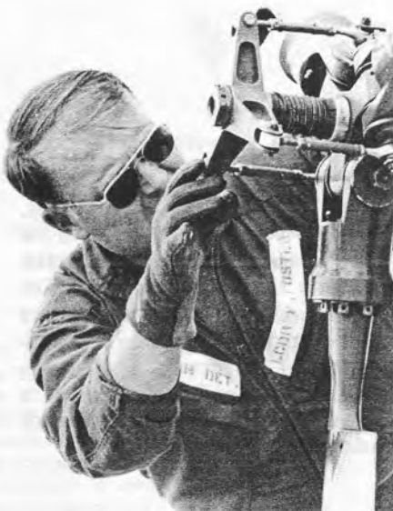
PREFLIGHT —USN photos by PH2 Ryden show Spartan Angel 028 undergoing last preflight check before taking off for the USS Lexington on historic flight. Above, Plane Captain ADJAN Kirby Sisco opens access doors to check engine, gearbox and other areas. Top right, Lieutenant Kearley checks the main rotor. Last photo, LtCommander Foster examines the tail rotor linkage.
