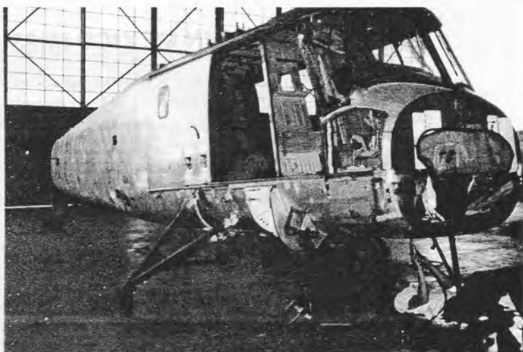
LINE READY —Stripped down to its "bare skin" and with all major components removed, fuselage is ready for structure PAR inspection. On completion, aircraft will move into modification station.
