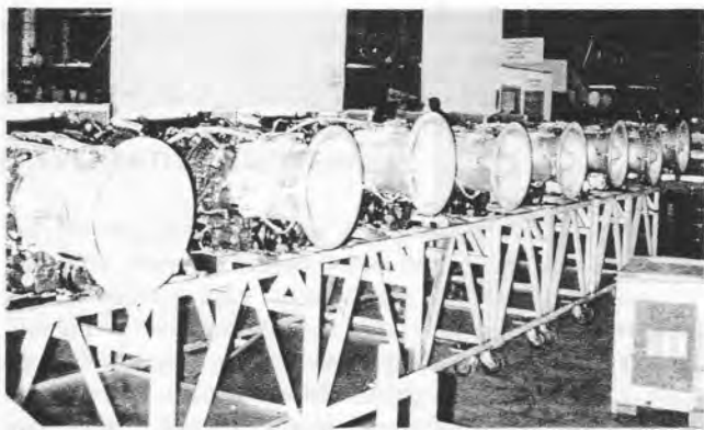
READY FOR INSTALLATION —Right and left hand engines stowed outside of engine build-up shop ready for installation.
