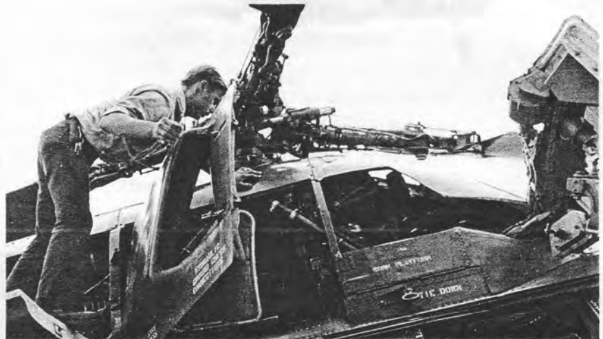
PREFLIGHT —USN photos by PH2 Ryden show Spartan Angel 028 undergoing last preflight check before taking off for the USS Lexington on historic flight. Above, Plane Captain ADJAN Kirby Sisco opens access doors to check engine, gearbox and other areas. Top right, Lieutenant Kearley checks the main rotor. Last photo, LtCommander Foster examines the tail rotor linkage.
