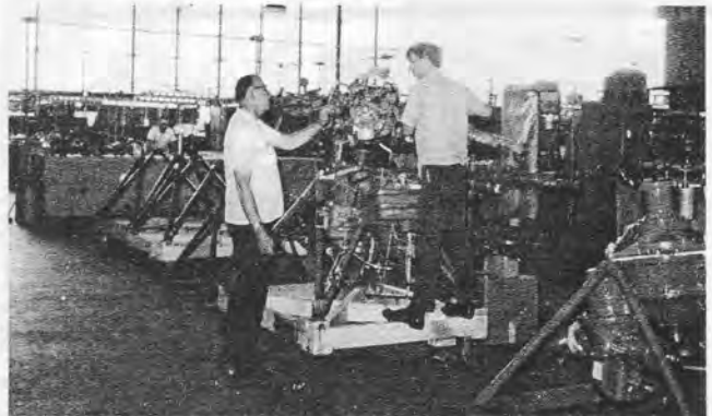
TRANSMISSION DISASSEMBLY —Transmissions being disassembled for further inspection and up-dating to latest configuration.
