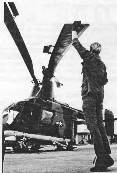
IT'S CALLED PEDRO —Returning from a fire suppression mission, the crew goes over the HH-43 very closely. Being inspected are the hub and composite rotor blades.
