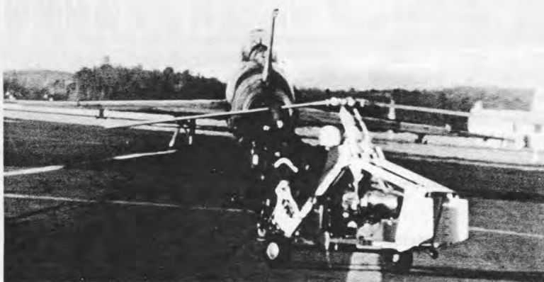
INITIAL FLIGHT —Preparations are made for first towed flight with prototype rotor. At left, SAVER waits behind an Air National Guard F-100 before receiving take-off clearance. Below, towed flight Jan. 10th.
