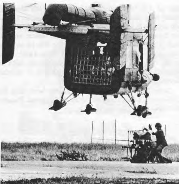
FSK HOOKUP —A fireman stretches out the door of an HH-43 Pedro to make sure the Fire Suppression Kit is properly fastened. The kit is designed to make a path to trapped crewmembers in the event of a crash, not totally extinguish a large fire.
