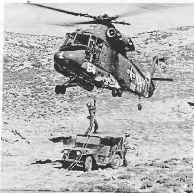
JEEP LIFT —At left, AMH2 Gary Labonte, assisted by ADJAN Gregory Paige, hooks up cable to the H-2's cargo hook preparatory to airlifting 2400-pound jeep to ship waiting off shore. At right, vehicle begins its over-water trip.
