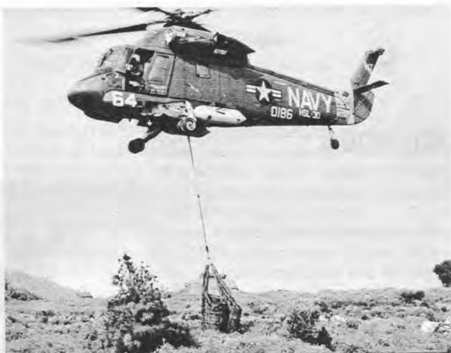
WORKHORSE —At left, HH-2D lowers 1300-pound load of fuel oil at a shore site. At right, helo is shown supplying a shore station. Tents, antennas, and other equipment in background, were all flown in by the H-2 crew.
