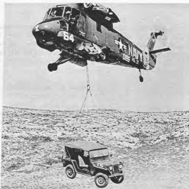
JEEP LIFT —At left, AMH2 Gary Labonte, assisted by ADJAN Gregory Paige, hooks up cable to the H-2's cargo hook preparatory to airlifting 2400-pound jeep to ship waiting off shore. At right, vehicle begins its over-water trip.
