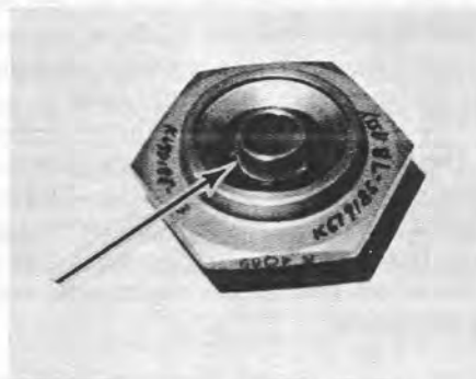
Sleeve protrudes 0.25-inch
