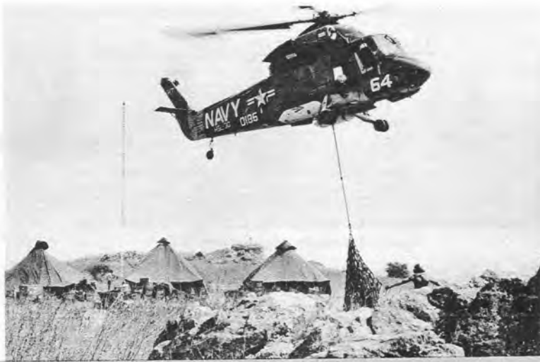
WORKHORSE —At left, HH-2D lowers 1300-pound load of fuel oil at a shore site. At right, helo is shown supplying a shore station. Tents, antennas, and other equipment in background, were all flown in by the H-2 crew.
