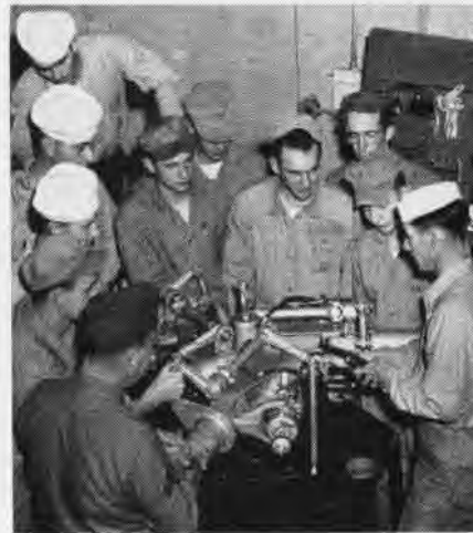
AT MEMPHIS mechanics school instructor Acord shows use of bearing puller for HO3S rotor
