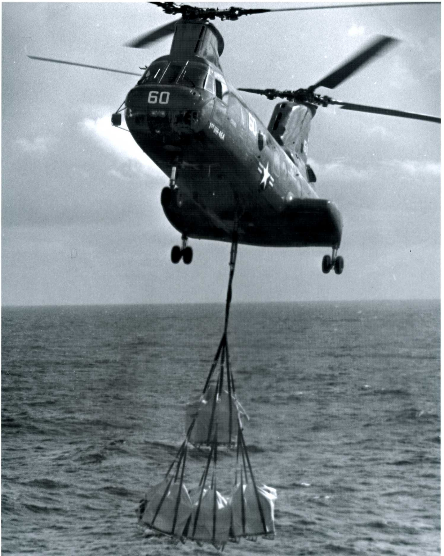
At the start of Vertical Replenishment on the West Coast the only cargo handling equipment was developed for inter-ship use and was not usable for VertRep operations, so we had to experiment with available items to get the job done. This rig proved to be unsatisfactory for Vert Rep.
