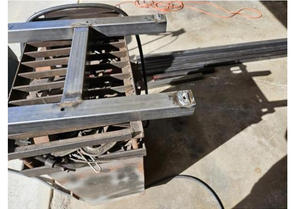
You will need a Chop/Cutoff saw to cut your steel and suitable welder to formally attach the three pieces of steel and weld in the weld nut inserts. The middle picture shows some weld nuts intended for stem caster installation on the underside of the frame and samples of the bolts used for the formal attachment of the seat to the top of the frame. Use actual Nylock nuts on those four seat attachments.
